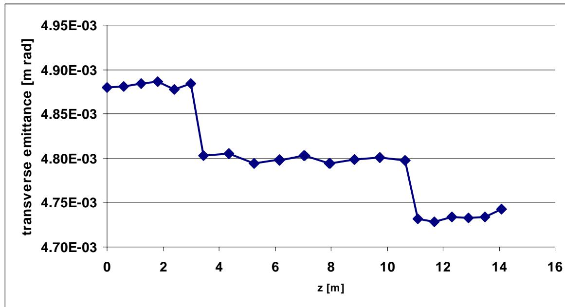
transv. emittance (r.m.s., norm.) vs z for 88 MHz cooling experiment (8 cav.) computed with *ICOOL* (50.000 particles)
