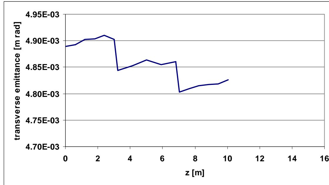
cooling performance of a system with only 4 cavities (50.000 particles)
