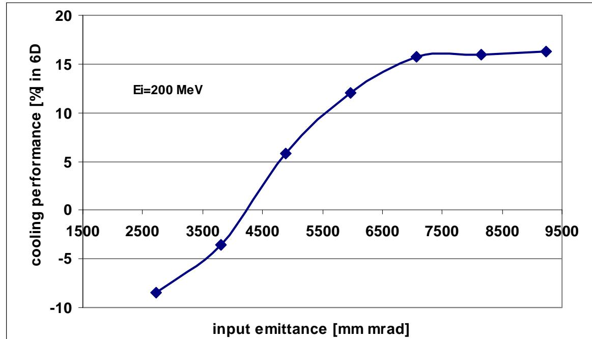
cooling efficiency is measured as number of muons inside
