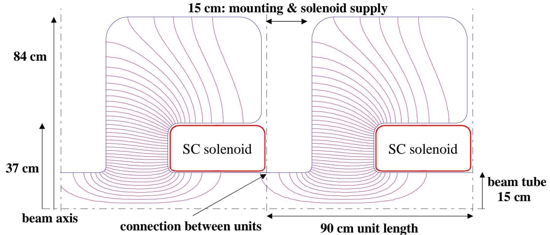
88 MHz cavities for muon cooling
