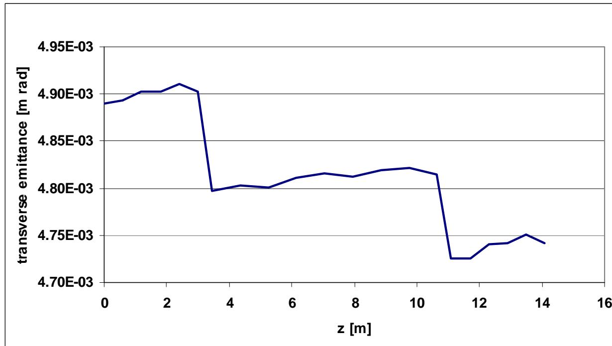
transv. emittance (r.m.s., norm.) vs  $z$  for 88 MHz cooling
