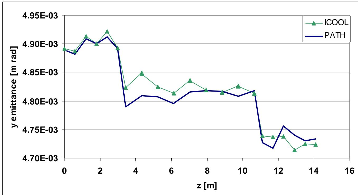
y - emittance (r.m.s., norm.) vs z for 88 MHz cooling experiment (8 cav.)
