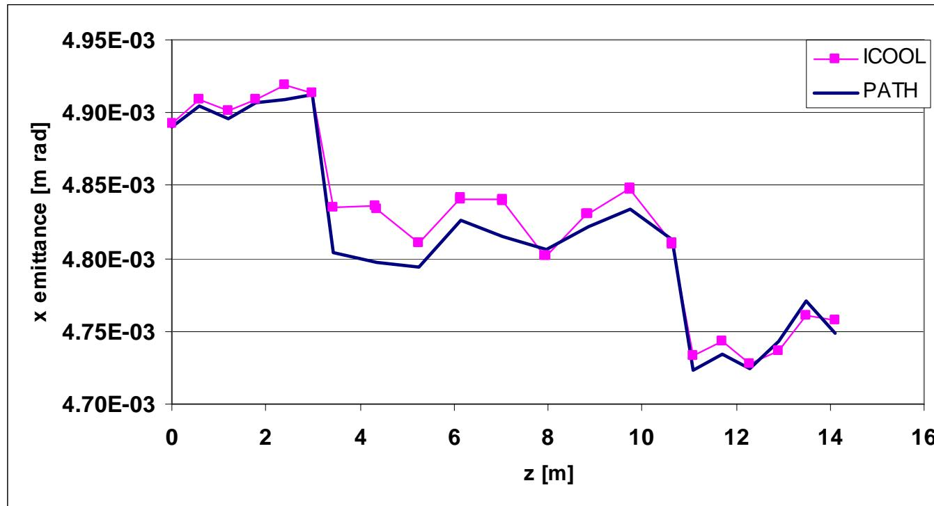
x - emittance (r.m.s., norm.) vs z for 88 MHz cooling experiment (8 cav.)
