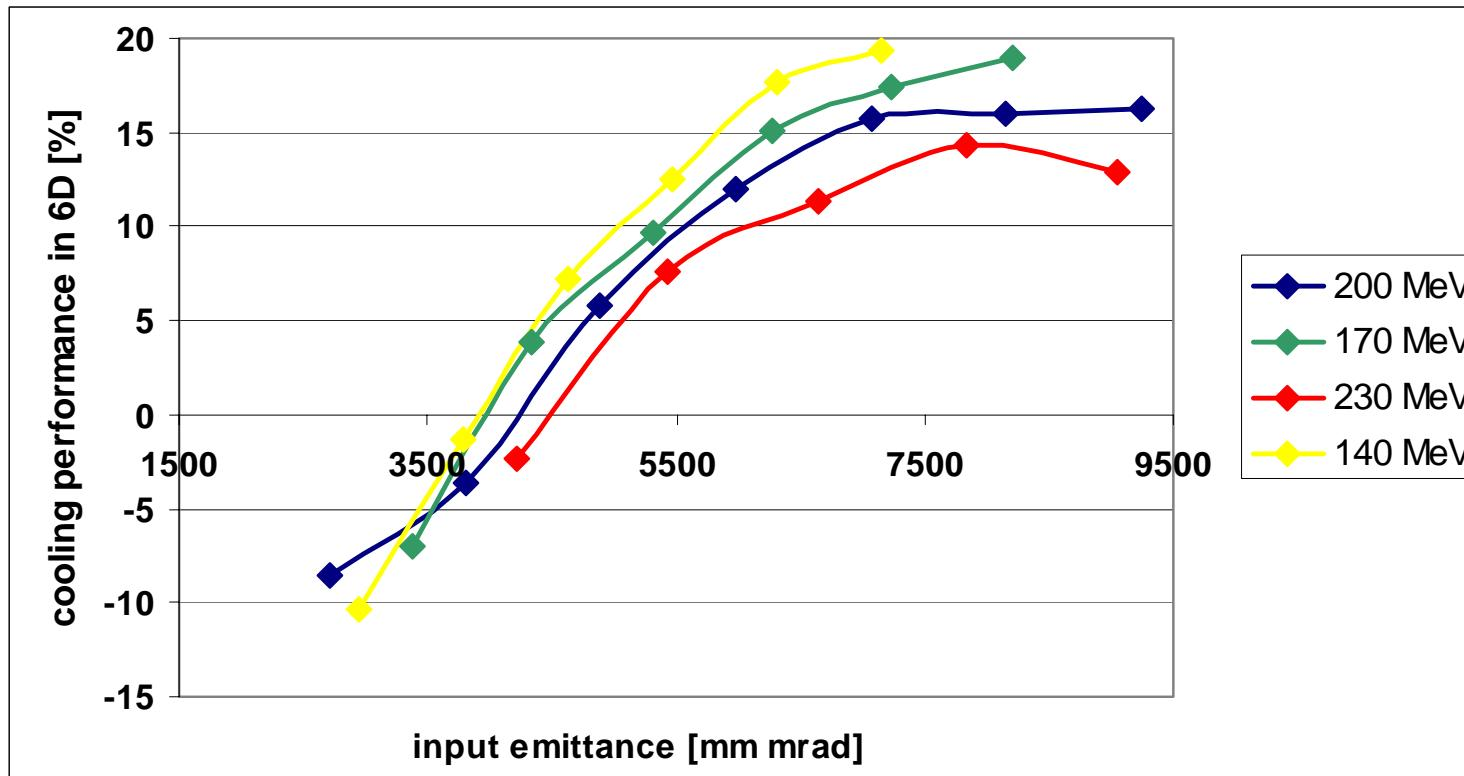
cooling efficiency for various input beam energies
