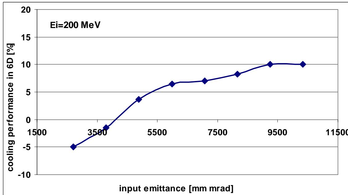
cooling efficiency is measured as number of muons inside
