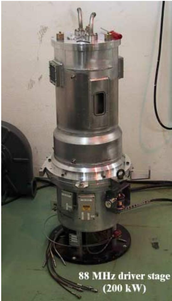
The RF chain up to 20 kW is assembled and will soon be turned-on. Next step will be to set-up the 200 kW driver stage which is already assembled
